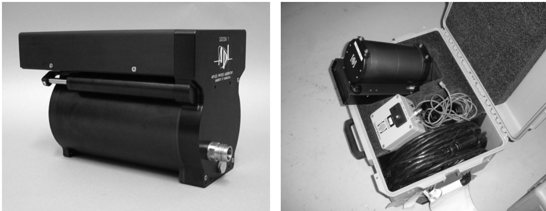
Figure 1: A standard unibody DIDSON transducer which weighs approximately 7kg and measures 171mm x 307 mm x 206 mm; b) A standard DIDSON accessory kit containing data cable, set-top box, Ethernet cables and the transducer. The operator additionally requires a laptop running DIDSON software to operate the unit.
